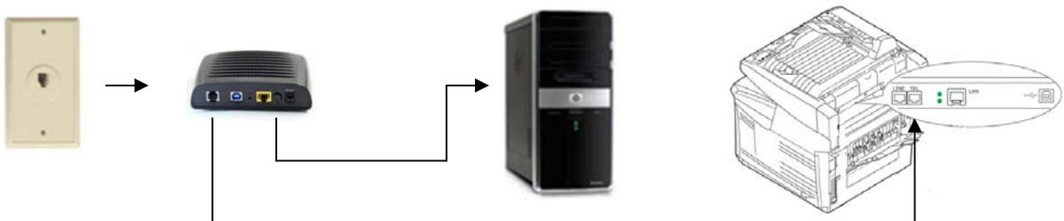
3. If the fax is connected to the same wall jack as the computer, and the router *does not* have a built-in DSL filter, the fax and computer connections will need to be split with a router. If the router does not have a built-in DSL filter (such as a Cisco 678 router), an inline filter needs to be installed between the fax and the router to ensure that the DSL signal is filtered from the printer connection (refer to the image below).
