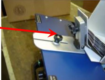
**STEP 6. You can raise and lower the back wedge ramp to find the optimum height for your stack.** To adjust the ramp height, loosen the locking knob on the back of the wedge upright and slide the ramp up or down to adjust. Then lock.
