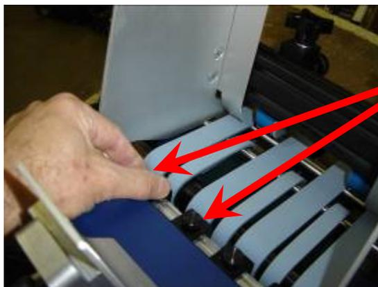
**With feeder running, loosen knob and move belt guide block by pressing against the block.**
