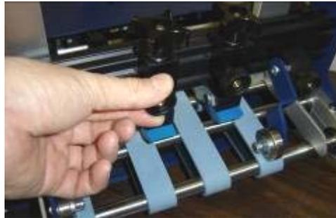
**NOTE:** When running wide stock (over 5" wide) you will likely be using two separators and at least three wide feed belts. When running narrow stock, you will be using only two wide belts and a single separator, positioned between them.
