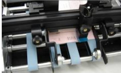
**These are just examples. AS-FDR12 feeders offer many different setup options with many different belt and separator configurations available. A bit of experimentation can be helpful.**
