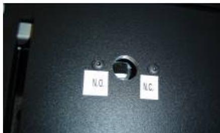
When the slide switch is in the N.C. position, the feeder will run when the host machine is NOT closing the leads attached to the AMP connector, OR when the interlock cable is removed from the feeder.
