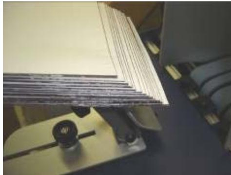
**STEP 2.** Slide this stack under the bridge, helping the stack to conform to the curvature of the paper guides and separators. Hold the rear end of the stack up off the belts in the hopper.
