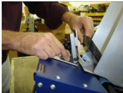
**STEP 5. Tighten the locking knob to secure the back wedge in place.**
